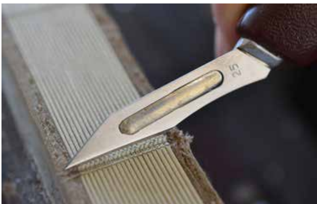
Using a scalpel to cut into the textblock at an angle
