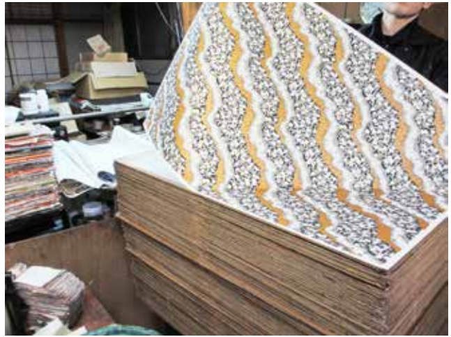
The last layer of ink having dried, the chiyogami is pulled off the board to which it was temporarily pasted. (Photo by Takao Moriki)
