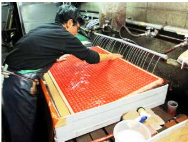
The paste resist on a sheet of katasome-shi is removed with water spray and gentle massage, exposing the white undyed areas.
