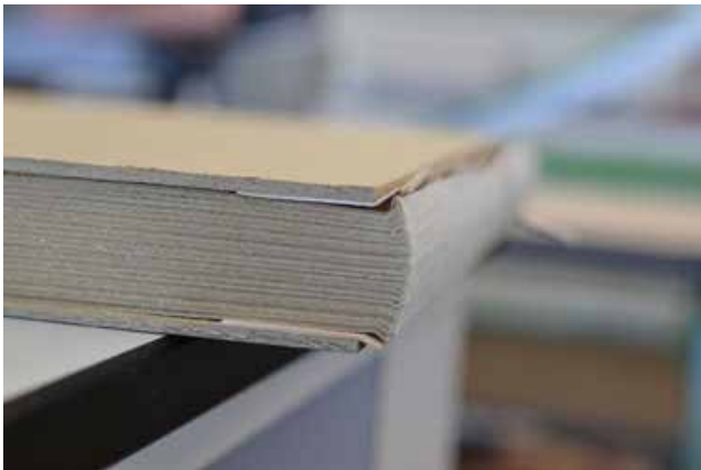
Thin card is folded up to fit the backing
