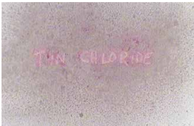
Tin chloride ink, on an alkaline paper, developed by spraying with a solution of cochineal.
