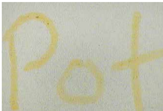
Potassium iodide after exposure to ultraviolet and ambient light for 24 hours.
