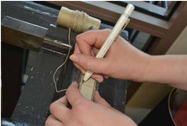
Marking the sewing stations using the cord that will be sewn around
