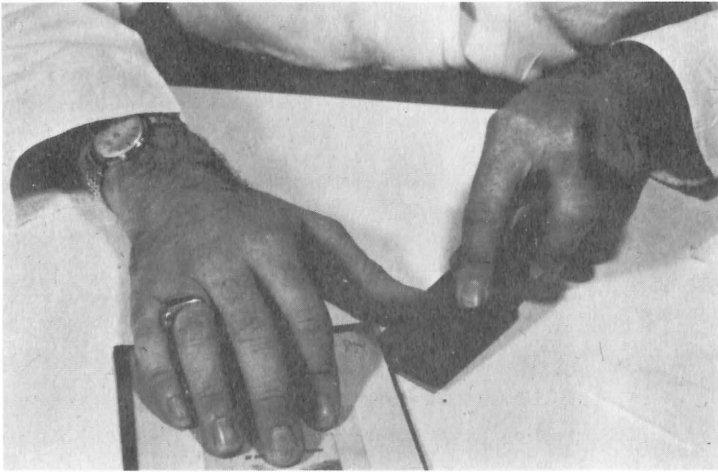
Figure 6. The endsheet is lifted from the board, using sweeping strokes with the leather paring knife.
