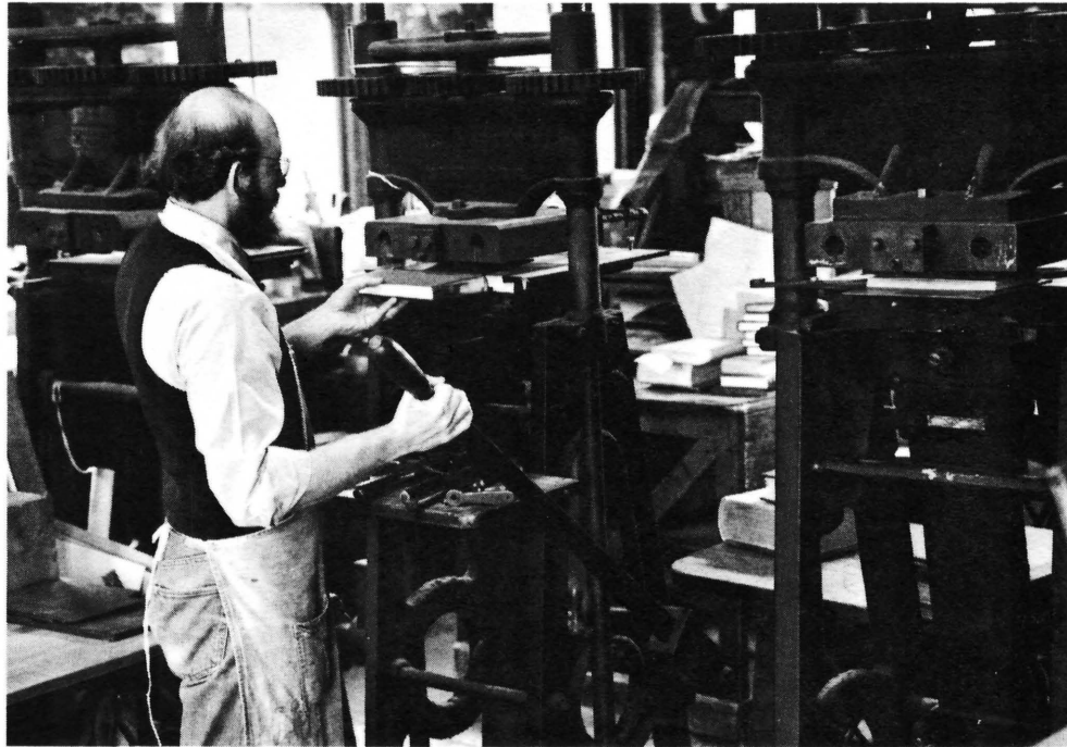
This picture of a section of the finishing area at The Harcourt Bindery shows three of the four gas-driven Imperial arming presses, used to stamp covers and doublures. The lever being pulled raises the bed of the press, in this case lifting the inside cover to the doublure die attached to the heated element. The wheel at the top raises and lowers the bed. (Photograph by Terry R. Harlow)
