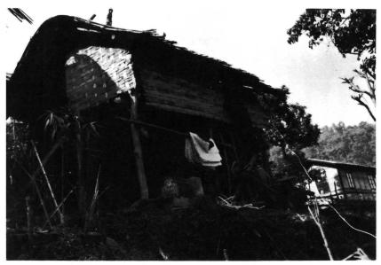
1. The papermaking house of Cho-sum, one of the four papermakers for the Rumtek Monastery in Sikkim. Finished sheets of paper are draped over the wooden pole attached to the house. The two baskets hold wood ash, used to produce a weak lye solution in which the Edgeworthia fiber is cooked.
