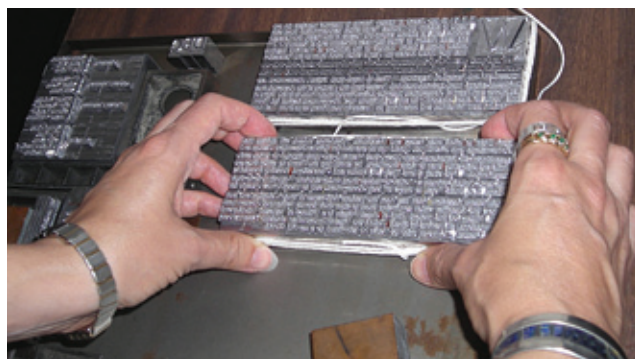
Transferring type from composing stick to galley for the historical re-creation, showing the first two paragraphs set on a 35 pica line.
