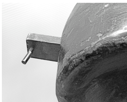
Safety pin for board shear counter-weight
