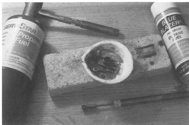
Figure 92 Propane torches and crucible with scrap brass on a fire brick.
