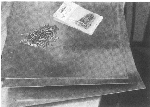
Figure 81 Sheet brass in various gauges, and brass escutcheon pins.
