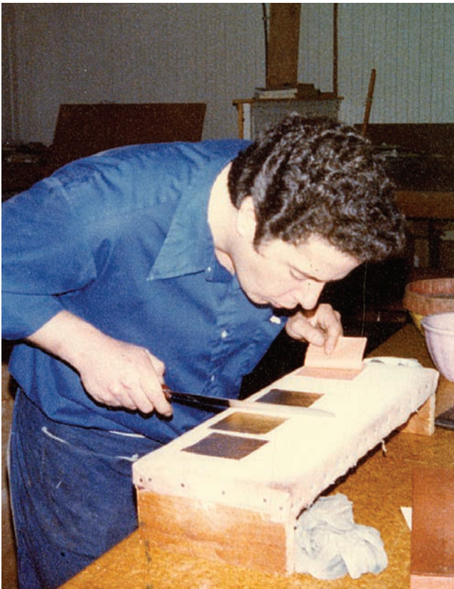
Fig. 9: Joe laying gold leaf on the gold cushion. Note that the gold cushion is long enough to comfortably lay out 4 leaves at one time.
