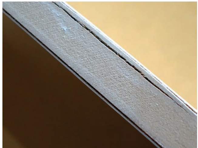
Fig. 8: The pull of the drying skin can delaminate the substrate. Photograph by the author.
