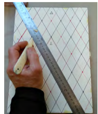
Figure 4-2. Pre-imprinting through a template.
