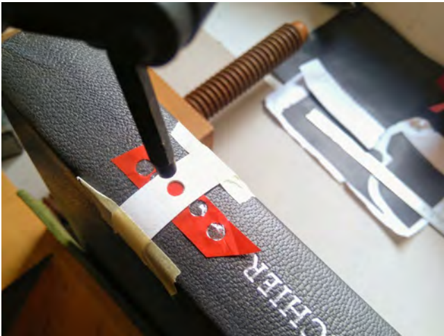
Figure 2-2. Template for tooling a dot.
