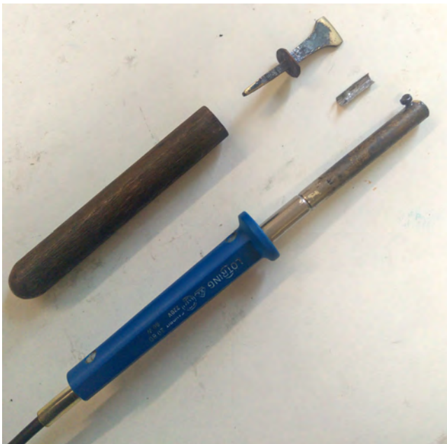
Figure 1-2. Soldering iron, sleeve, and tool head.
