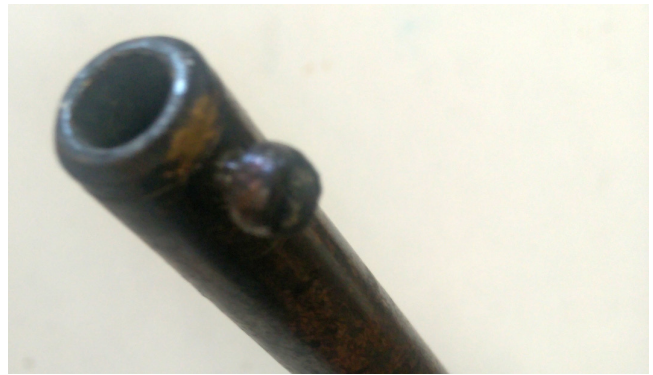
Figure 1-3. Opening at end of soldering iron. Older, fixed temperature tools.
