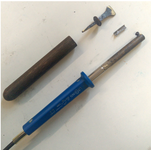
Figure 1-2. Soldering iron, sleeve, and tool head.
