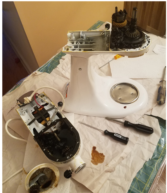
Lockdown work, re-greasing the KitchenAid.
