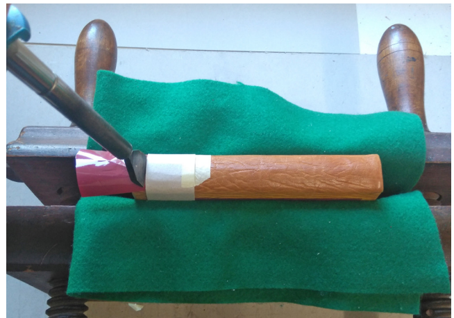
Figure 6-1. Simple card template for line tooling.
