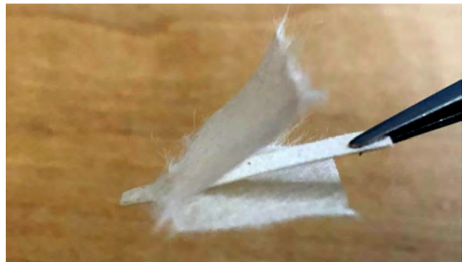
A composite support extension made with parchment and kozo tissue.
