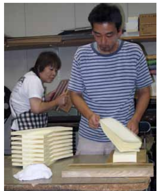
Fanning glued-up accordion-folded books to separate pages
