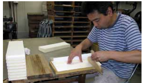
Pasting edges of folded sheets, placed back to front, cut edge to fold
