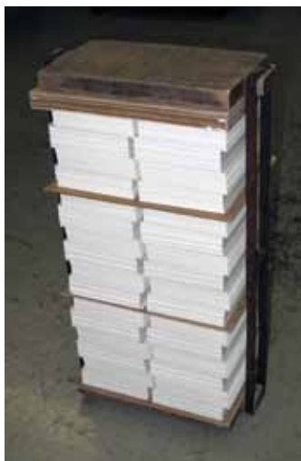
Traditional book press holding partially glued-up text blocks
