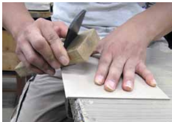
Forming a beveled edge using a planer while books are in a pile
