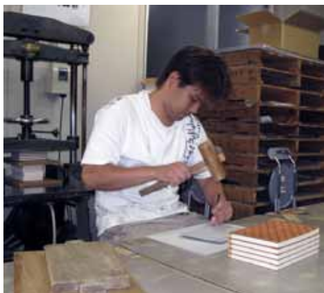
Pounding holes with hammer & awl into template prior to using it for placing holes in book
