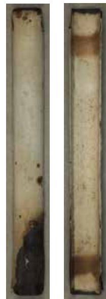
Fig. 2 The outer and inner faces of the metal spring covered in paper. The stains on the inner facing paper are from contact with leather tabs lining the spine of the text.
