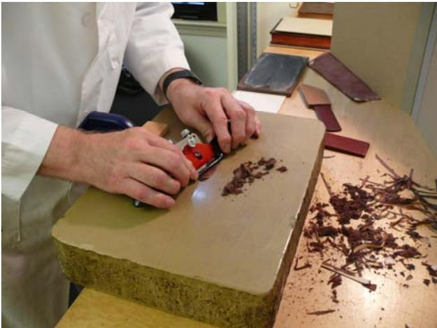
Thinning and shaping leather with a spokeshave takes some practice, although spokeshaving is easier to do than to describe. Stand while spokeshaving, in order to be able to see the front of the tool. Use a clamp and wooden board to hold the leather in place on a litho stone. Adjust the blade so that very little is extended beyond the base. It is surprising to students exactly how little of the blade need be exposed. Test if there is too much blade showing by placing the
