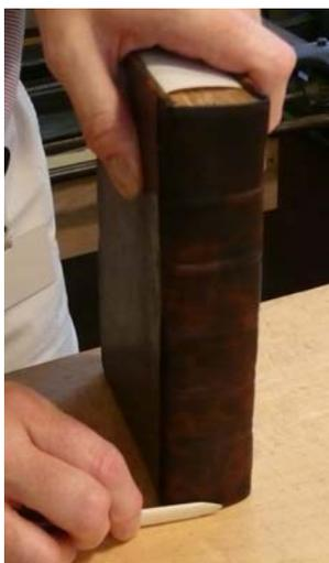
Place the book on the bench, pressing down and tapping lightly on the spine at the headcap with a folder. To form the headcap, lightly press down and move the book slightly forward and backward. If there is too much leather in the headcap area, pushing toward the spine will draw the headcap in over the head of the book; pushing away from the spine will draw the headcap away from the head. This is a very subtle movement, almost invisible to anyone watching.
