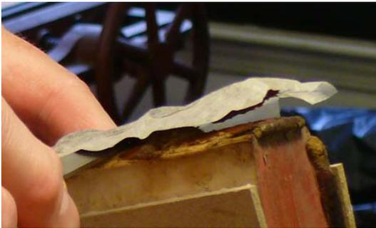
It may be necessary to lift from both sides of the spine. The small lifting knife is good for beginning the lift, and for lifting around raised bands, but switching to a broader lifting knife is useful for wide or long spines. Make sure to retain the entire headcap, if one remains, although this is rarely the case. If the spine breaks into pieces during the process, store the pieces along with a piece of paper
