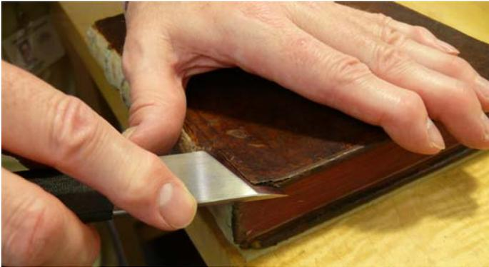
Make several more passes with the knife at a much lower angle, lifting further with each pass. Slice right through the covering leather at the edge of the board. If there is tooling or decoration on the board edge, it may be lifted separately, so that the new rebacking leather can be inserted under the decoration. This little piece of edge leather is usually so
