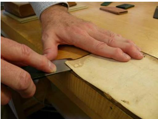
For unattached boards, the pastedown is lifted along the entire spine edge to accommodate new hinges. Begin the lift under the existing turn-in leather. Either a curved or straight knife may be used for this; sometimes one works better than the other, depending on the paper. Insert the knife 1/8", lifting down along the entire edge. Lift in several passes, extending the depth with each pass. Try not to lift any of the board; the idea is to lift the turn-in leather and the paper only.
