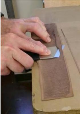
The second pass of the knife is done with the edge of the knife angled slightly away from the edge of the leather, and at a much lower angle. A third pass of the knife may or may not be needed, before spokeshaving, depending on the thickness of the skin.
